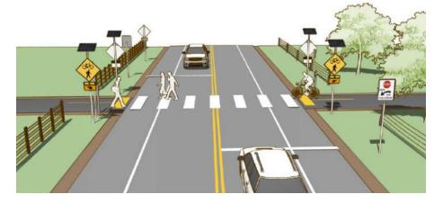
Providing comfortable crossings where trails or bikeways cross roadways can make the difference in completing the network and providing a continuously safe experience. The map on page 53 highlights several locations where mid-block crossings are proposed. In most cases, further study and engineering analysis is needed to determine the appropriate crossing type at each location. The following graphics illustrate various types of crossings that are likely to be considered in Osawatomie.
