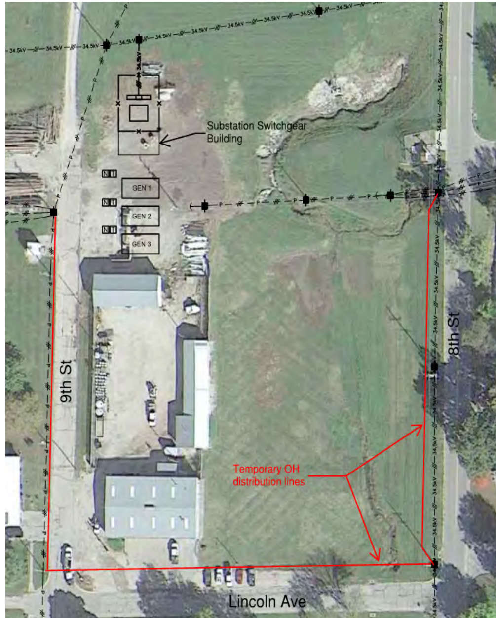
Figure 7: Proposed Substation Layout
