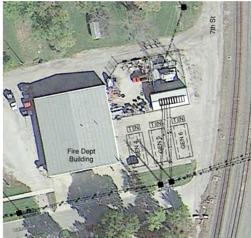
Figure 3: Proposed Generator Layout at 7 th St Substation.
