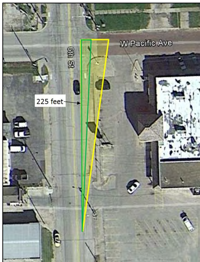
Figure 11 - Approximate Recommended Intersection Sight Distance for Westbound Left Turns (6th St. & W. Pacific Ave.)
