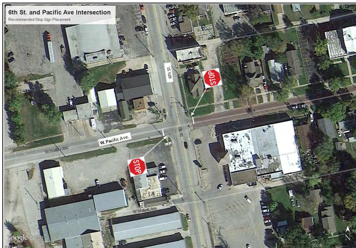
Figure 13 - Recommended Stop Sign / Stop Line Placement at the 6th and W. Pacific Intersection, Osawatomie, KS
