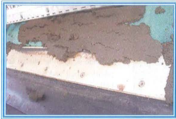
The TRITAN discharges a biosolids cake with a solids concentration of 15 percent to 20 percent.
