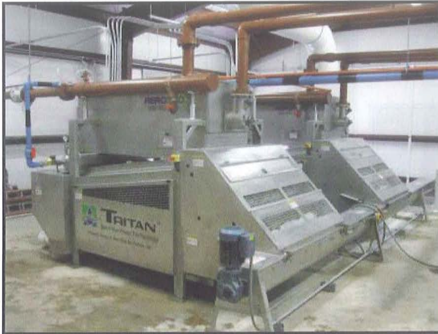
The TRITAN dewatering belt press provides three belt performance with single belt tracking.
